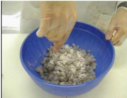
Apply powder in the bowl or mixer, and mix 4-5 mins. to coat all surfaces
